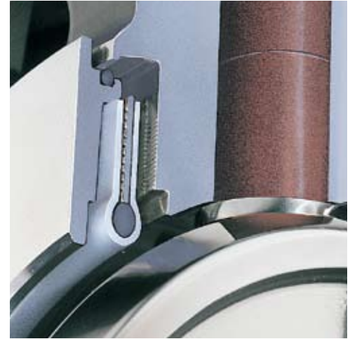
PFA/Viton® A energized seat provides positive, bidirectional shut-off with long cycle life on low pressure and vacuum, and high ΔP services. (See page 21 for more information about seating.)
